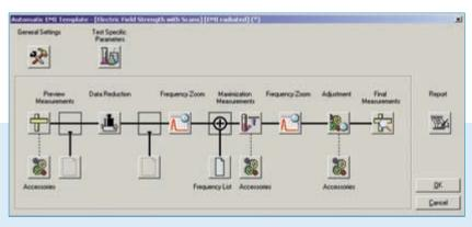
Test template of an automatic RFI field strength measurement with the setting elements for preview measurement, data reduction, optional maximization of the critical frequencies with positioning of accessories, final measurement and report generation.
